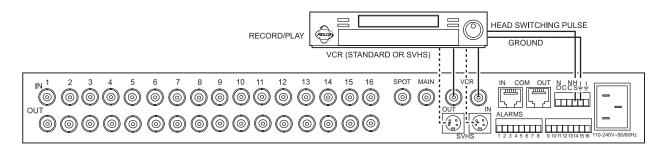
Figure 6. VCR Wiring Example
